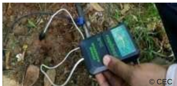
Measuring moisture to plan irrigation schedule
